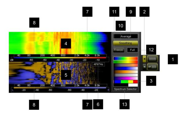
The spectrogram views are turned on using the spectrogram View Selector controls [1]. The adjustable parameters are displayed on the Edit Control Panel [3] which is accessed via the adjacent Edit Selector control [2].
