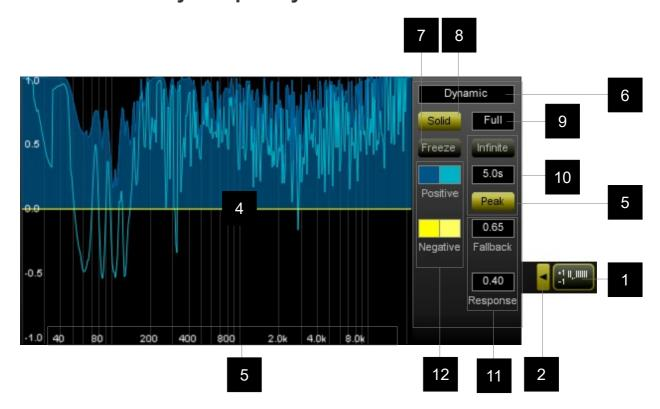
The correlation meter view is turned on using the correlation meter View Selector control [1]. The adjustable parameters are displayed on the Edit Control Panel [3] which is accessed via the adjacent Edit Selector control [2].
