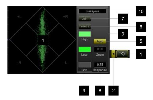
The Vectorscope view is turned on using the Vectorscope View Selector control [1]. The adjustable parameters are displayed on the Edit Control Panel [3] which is accessed via the adjacent Edit Selector control [2].
