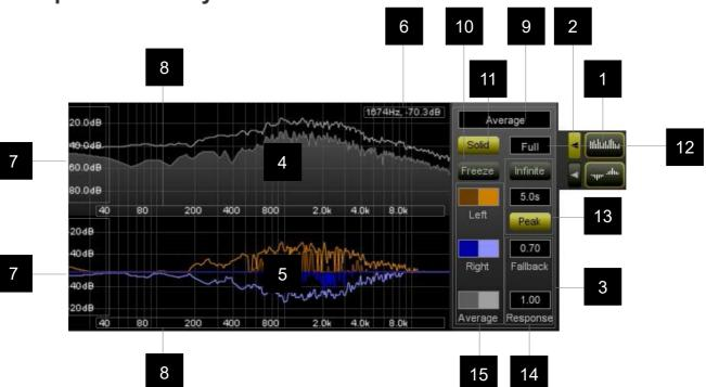
The spectrum analyser views are turned on using the spectrum analyser View Selector controls [1]. The adjustable parameters are displayed on the Edit Control Panel [3] which is accessed via the adjacent Edit Selector control [2].
