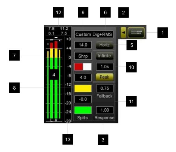
The level meter view is turned on using the level meter View Selector control [1]. The adjustable parameters are displayed on the Edit Control Panel [3] which is accessed via the adjacent Edit Selector control [2].
